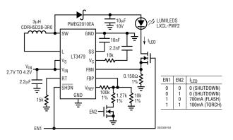
Figure 4. The LT3479 Boost Regulator Delivers 700mA Constant-Current to the LXCL-PWF2 High Voltage Luxeon Flash with 85% Efficiency and Output Disconnect
